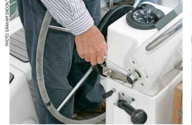
For security, give the engine a solid blast astern to get the anchor set
