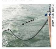
If the rope snubbers are at their limit, Tom Partridge adds rubber snubbers to absorb the snatch
