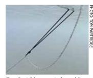
Tom Partridge uses twin snubbers for double security, giving a less anxious ride at anchor
