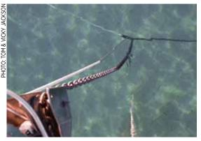
A Bahamian moor: two anchors laid off the bow, on two cables joined by a snatch block. It's secure, but hard to lav and recover
